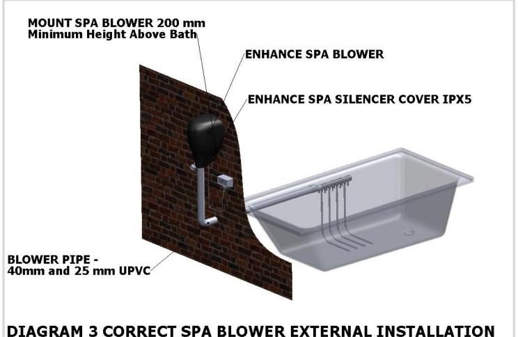
DIAGRAM 5 CORRECT SPA BLOWER EXTERNAL INSTALLATION
